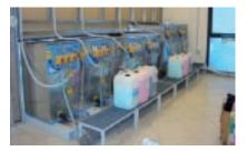
IMESA washing machines may be connected to detergent pumps; the customer needs only to choose the wished program, the machine does all the rest. Washing programs are created optimising softener, detergent and disinfectant without any waste!
